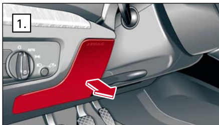
Fuse box – left-hand drive (steering wheel left)
