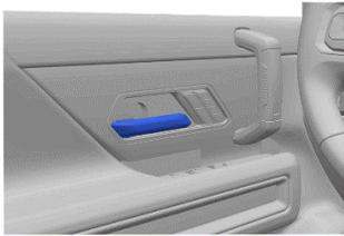
If the doors remain locked, pull **twice** on the inside door handle to gain access to the occupant at each seating location.
