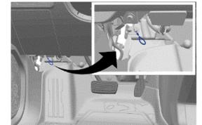
3. Remove the front compartment sight shield.
