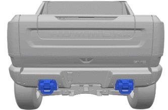
The vehicle may be equipped with two optional rear tow hooks to pull the vehicle onto a flatbed carrier from a flat road surface.
