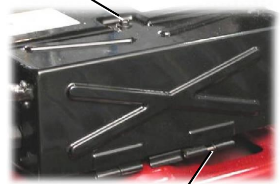
Hinges attached to the battery hold the cover in place
