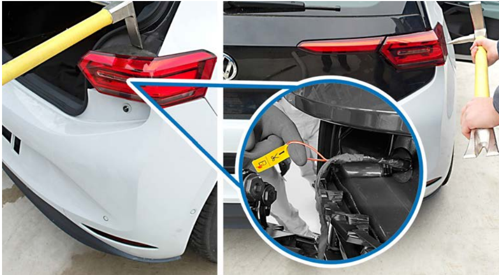
Variant 2: Cut-off point in the rear of the vehicle behind the right tail light cluster from the start of 2021.
