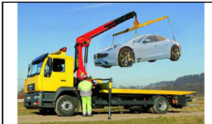
Figure 10C. Hiab recovery (for completely immobile vehicle)
