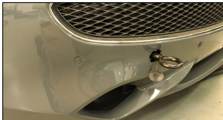
Figure 11.I. Recovery eye should be in horizontal position before attaching winch cable
