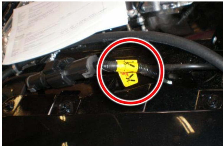
Figure 8A. Right-side low voltage disable location
