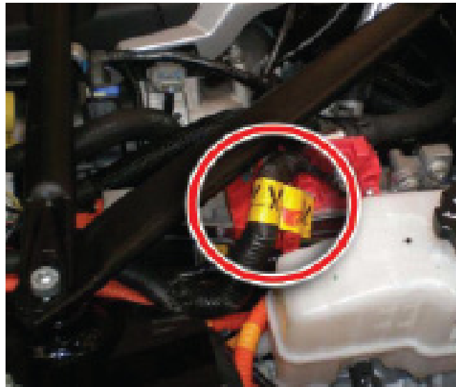
Figure 8B. Left-side low voltage disable location
