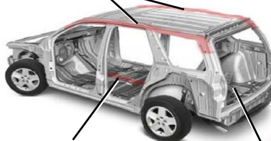
**DO NOT CUT HERE.** Channel beneath the vehicle contains intermediate 36v electrical wires
