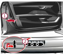
Remove the cover Release separation point
