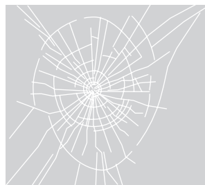
< Broken Laminated Glass >
