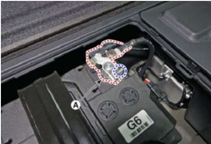
4-2. Turn the ignition switch OFF and disconnect the auxiliary 12 Volt battery negative (-) terminal (A).
