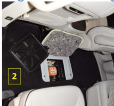
2 Second: Unbolt the cover panel over the Service Disconnect.
