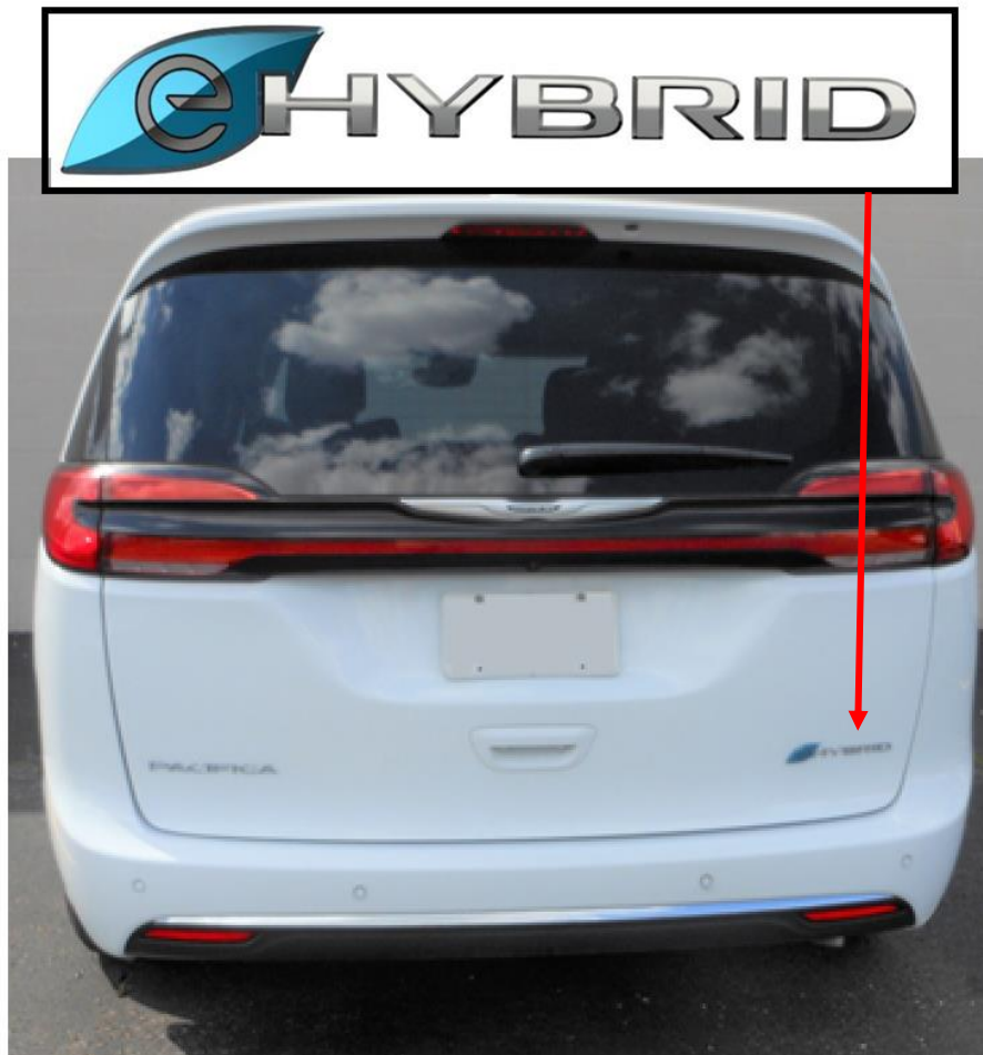
Unique badging on lift gate on the passenger-side rear.
