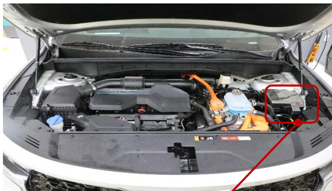
Engine room fuse box
