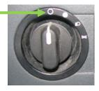
3. Open the curb-side rear fender at the rear of the bus and turn the 12/24V emergency disconnect switches to the OFF position:
